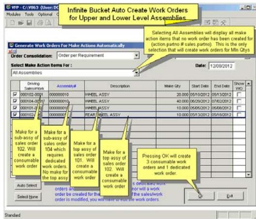
pc/MPR versions 8.63D and higher allow users to automatically create work orders for both top level assemblies and or lower level sub assemblies.
